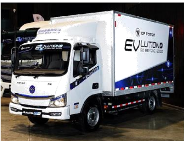
Auman EST iBlue280 Battery 282 kWh Driving range 200 km/charge Motor 360 kW
